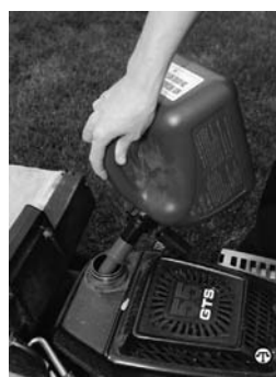
Don't be fuelish-Use only E10 or lower fuel in any lawn and garden equipment.
