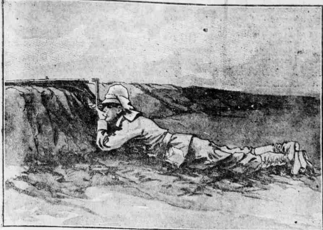
An English clergyman has invented a device which enables a marksman to aim over walls, ramparts, etc., without exposing himself to the fire of the enemy. It is called the hyposcope. The device consists of an arrangement of mirrors in a vertical tube which reflect the sunlight and save the shooter from exposing his head to look along the barrel. At four times in thirty-five shots.
