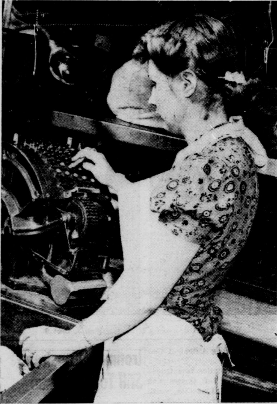
MRS. VIRGINIA QUINN shown operating machine which stamps laundry number on items of clothing. Looks like an adding machine, but isn't. — Signal Corps Photo.
