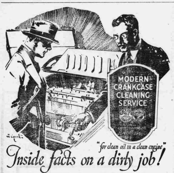
VOUR ENGINE requires an internal bath frequently. Road dust, carbon from the combustion chamber, and fine particles of metal worn from the bearing surfaces get into the lubricating oil in the crankcase. All this dirt circulates with the oil through the engine. If it isn't drained out regularly there's bound to be excessive wear and tear.
