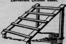
Select two four inch pieces six feet long. Lay them parallel and nail five crosspieces, three feet long and three inches wide, to these. The legs may be made of 2 by 4 stuff the desired length. By means of long spikes secure them to the parallel pieces. Place this in roosting quarters for chickens and they will soon be perching upon it at night .- Iowa Homestead.
