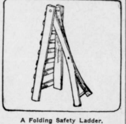
A Folding Safety Ladder. by four-inch stuff. Bolt the two supports together in the middle. Spread the lower ends as shown and use a rod for the connection at the upper end. The longer the ladder, the heavier the uprights should be. Such a ladder can be folded and carried with ease.
