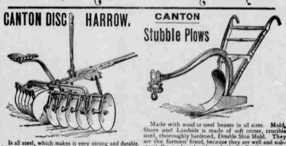
Is all steel, which makes it very strong and durable. It is simple in construction and has less parts to wear than any Disc made. The chilled journal bearings are entirely dust-proof and can be easily oiled. There is absolutely no end thrust to wear on the bearings.
