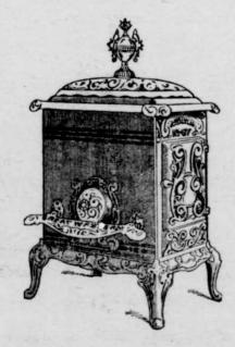
The body is made of genunine planished iron and is protected by a cast lining, the front section of which is so formed that the draft admitted by the screw damper is carried downward nearly to the stove bottom. The door opening is very large and is provided with a smoke curtain. There is a check damper under the pipe collar to be used in keeping fire at night. Heavy cast ribs to hold a layer of ashes. We will be pleased to show you the many good points of this wonderful heater.
