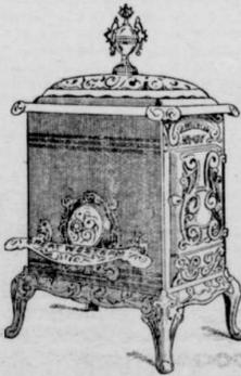
The body is made of genuine planished iron and is protected by a cast lining, the front section of which is so formed that the draft admitted by the screw damper is carried downward nearly to the stove bottom. The door opening is very large and is provided with a smoke curtain. There is a check damper under the pipe collar to be used in keeping fire at night. Heavy cast ribs to hold a layer of ashes. We will be pleased to show you the many good points of this wonderful heater.
