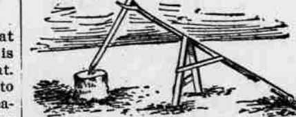
RIG FOR SHARPENING POSTS.
