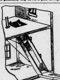
REGULATES SPEED OF THE BARREL
