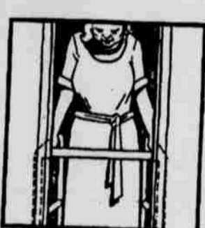
Remake the doorways at least 32 inches wide. If the door is not essential, remove the door.
