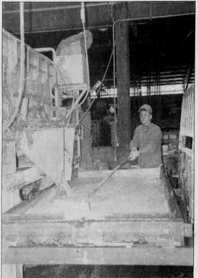
Jim Mehlberg works slurry as it is poured into frame.
