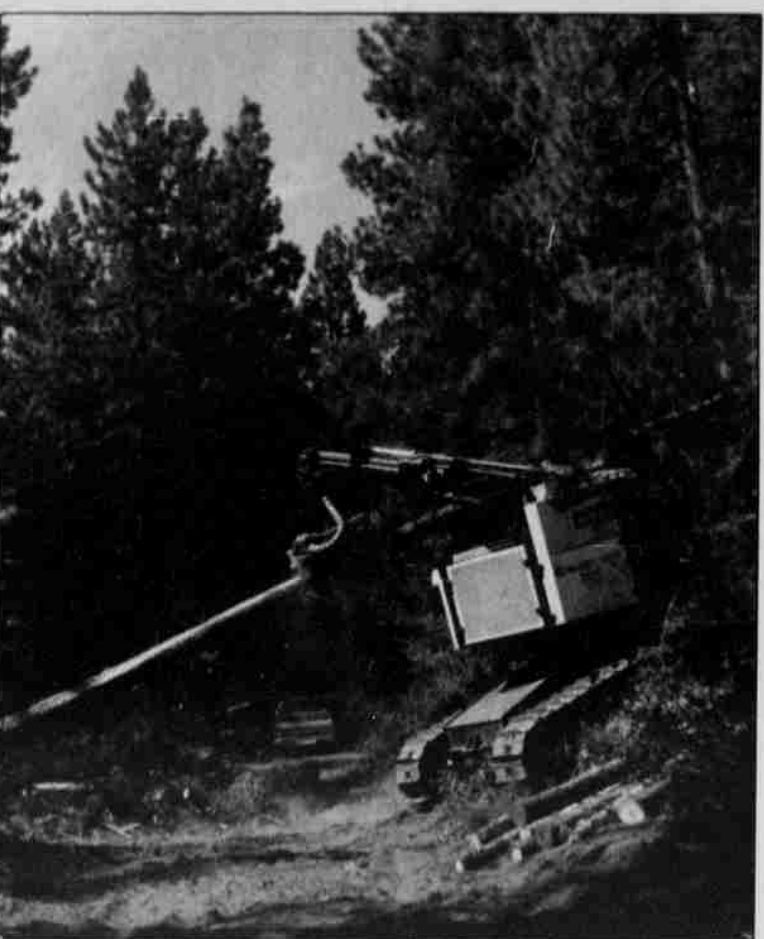
Automatic tree cutter and limber prepares trees for loading.
