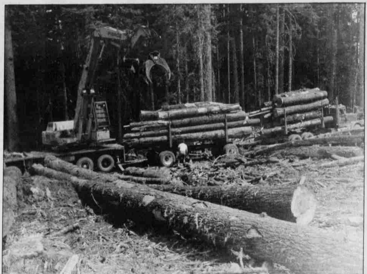
A Smith-Greene shovel loads a truck with cull logs headed for a chipper in The Dalles.
