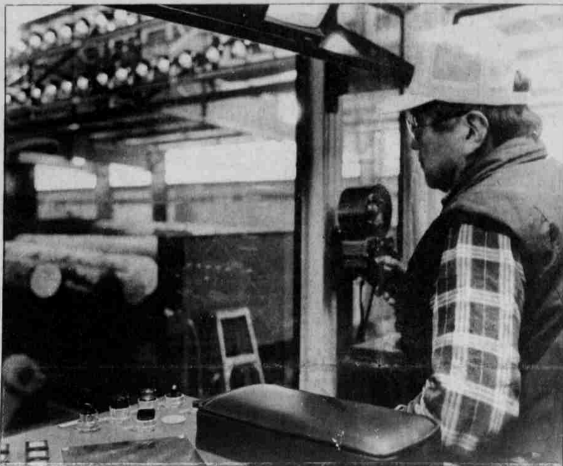
Earl Squiemphen operates the End Dogging Log Feed system at the new small log saw mill. The EDLF is the primary log breakdown system at the mill.
