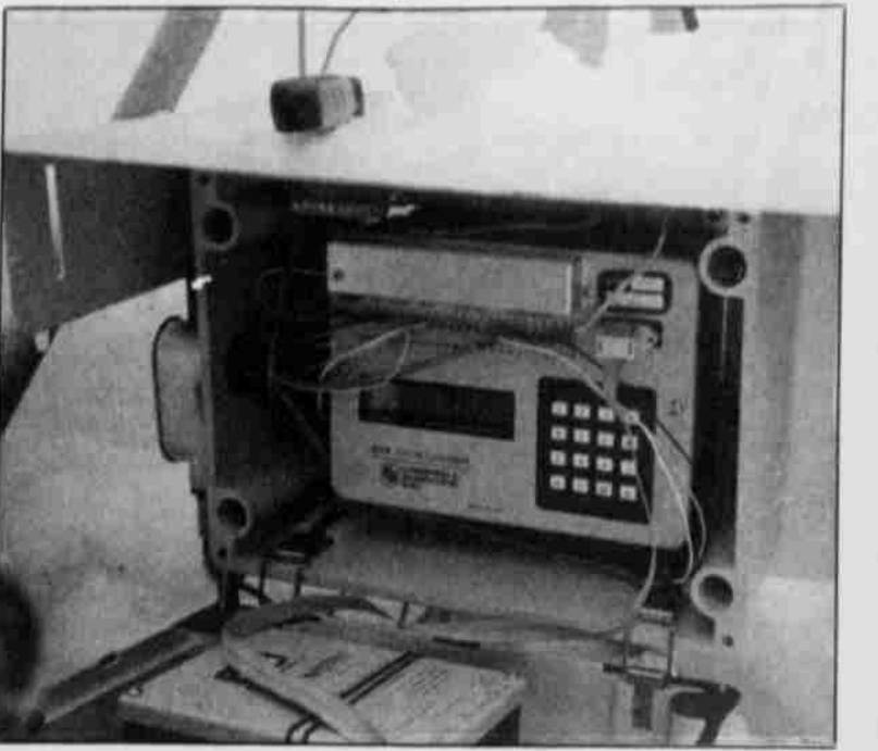
Microcomputer instruments are used collect rainfall and weather data at various places on the Warm Springs reservation.
