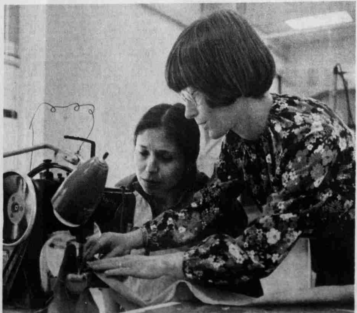
Apparel Industries manager Dorothy Pedersen instructs Roxanne Spino on use of machine to make felled seams.
