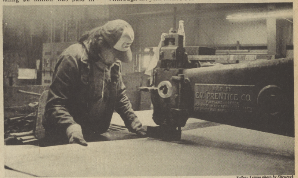
Kirby Heath operates a Reimann machine while patching veneer at Warm Springs Forest Products Industries.
