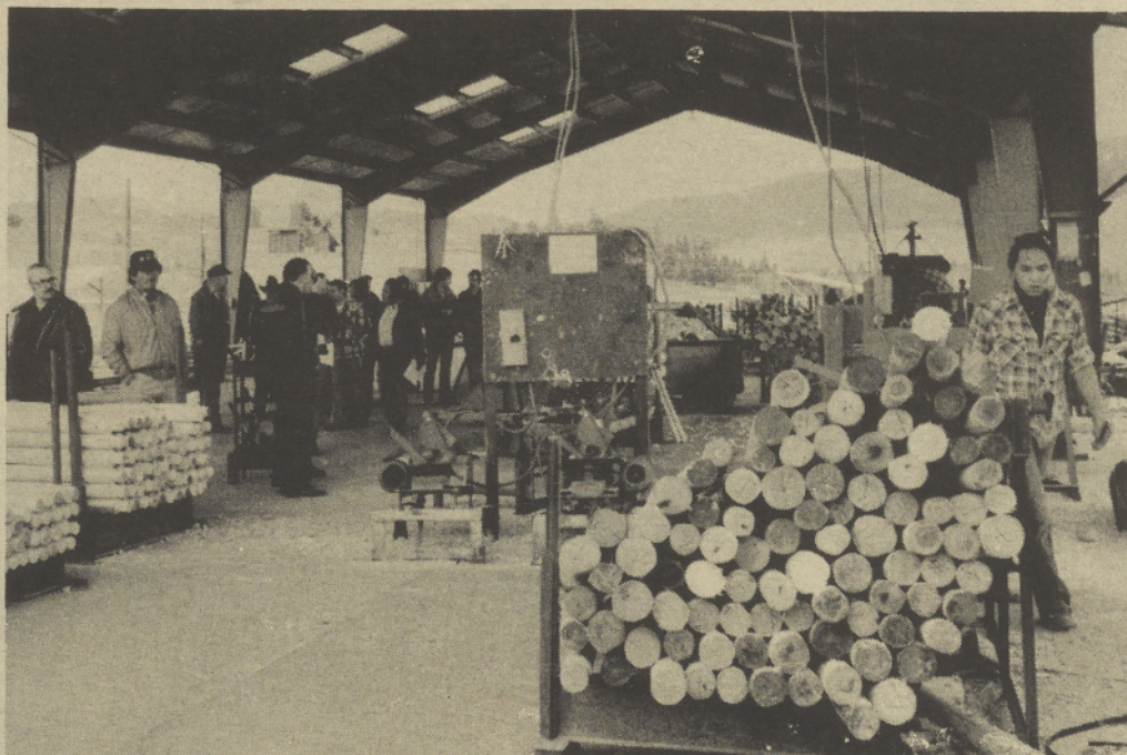
Spliyay Tymoo photo by Behrend The Flathead Post and Pole enterprise located in Dixon employs about 300 full and part time employees. The operation produces posts, poles and fencing material. Northern Lodgepole Pine is used for all materials.
