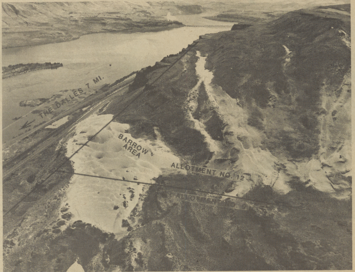
The sand dune marked Barrow's Area located seven miles east of The Dalles is slowly moving towards the Columbia River. The fine particled sand continuously has to be removed from the highway and railroad tracks to ensure safety. The Confederated Tribes of Warm Springs has donated rock from sections owned by the Tribe and its members to stabilize the dune. Work will begin this summer.
