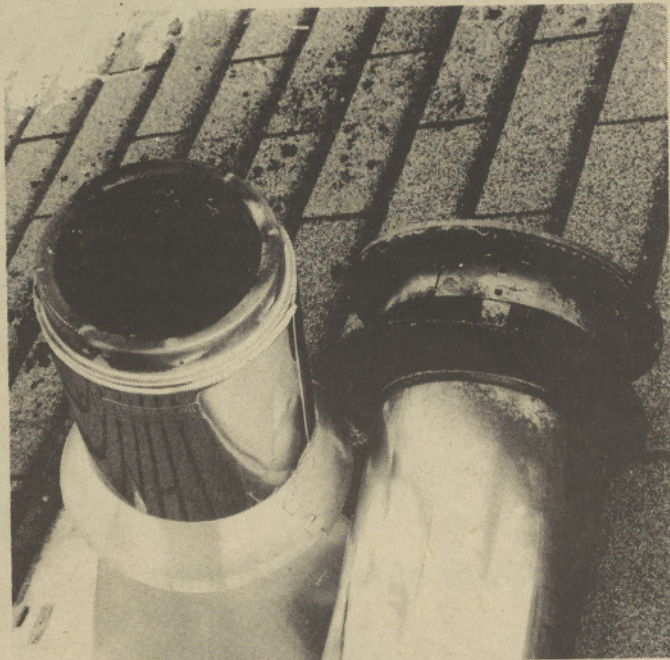
Creosote build-up contributed to setting this senior's home on fire. Flues should be kept clean.
