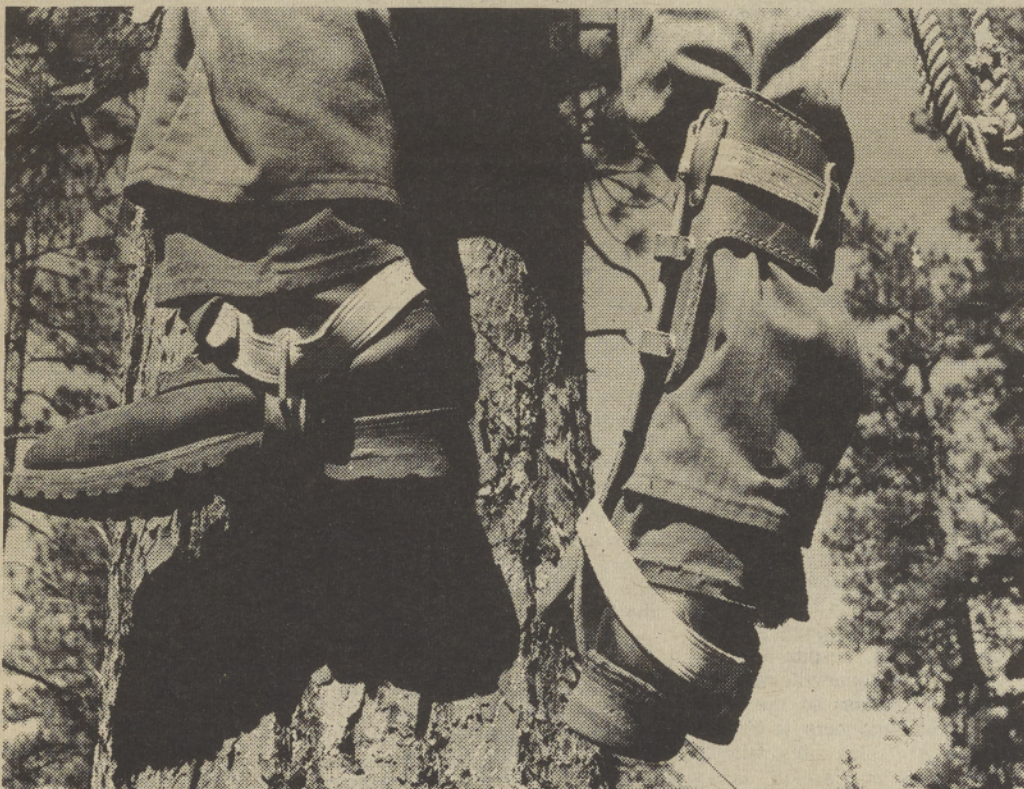
SPURRED ON — One way of getting up a long tree trunk is to strap on spurs and walk up, a skill that takes time to master. The pain involved is not so much in the feet and calves but in the arms, which had to do a bit of hoisting. The rope dangling in the upper right is slung around the tree and attached to the forester's harness while he is picking cones. CDS Photo
