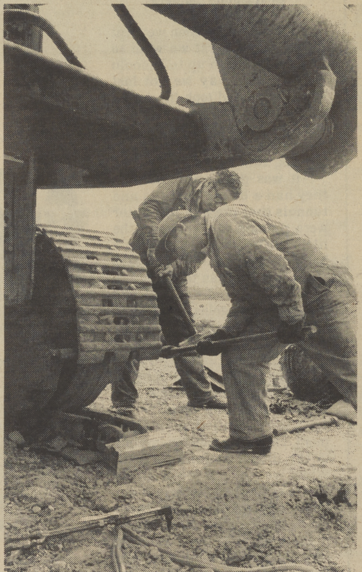
Albert Comedown, like all the loggers, does as much repair work as he can right in his own yard. Just before the beginning of the season Albert (right) and his woods boss Don Waldrip repaired the track on a cat. CDS Photo
