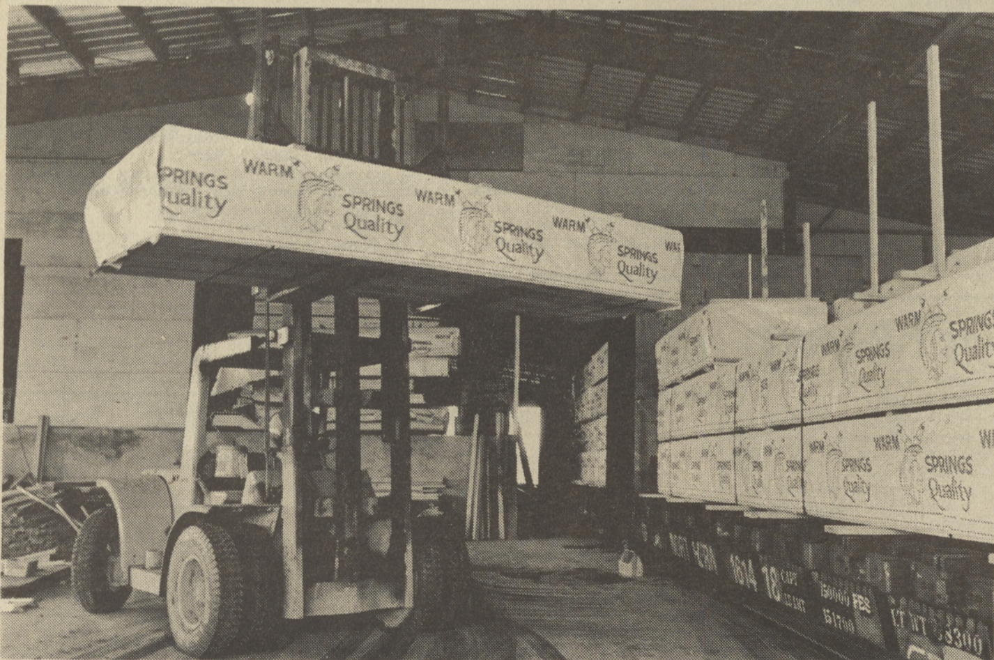
Lumber delivered in unitized packages is more attractive to markets and more efficiently loaded. At WSFPI's expanded loading dock in Madras, forklifts hoist packages of lumber onto flatcars or boxcars from track level. The old platform (rear) was designed for loose loading, an outdated method of handling. Plans are to extend the track and concrete slab to allow for more shipments each day.
