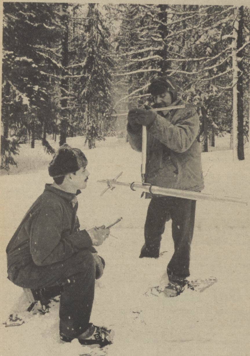
After measuring the snow depth, Miller weighs the core sample on scales suspended from a ski pole while Luther records the reading. Both wear snowshoes, not only to keep from sinking into the snow, but so they won't disturb the snow or cause future readings there to be inaccurate. Sandy Rangila Photo
