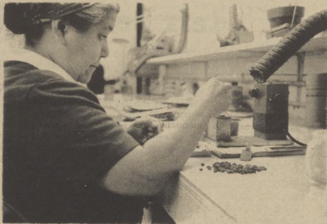
The exhaust hose (right) sucks up excess smoke and fumes as Maxine McKinley is tinting leads for better electronic contacts. Maxine is one of the original trainers and has been with the plant 8½ years.
