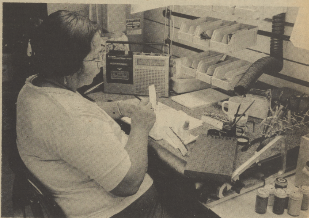
Edith Kalama puts the finishing coat on some toroids with a paint brush, then allows them to dry. After two hours, the toroids are popped into the oven for two hours, then all that's left is the packaging for shipment.
