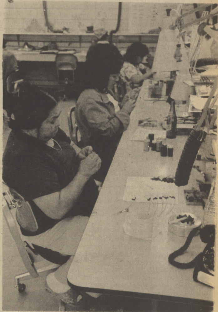
Marjorie Danzuka is winding red and gold insulated wire onto the toroids while JoAnn Moses paints the color coating onto the toroids, as is Linda Allen in the background.
