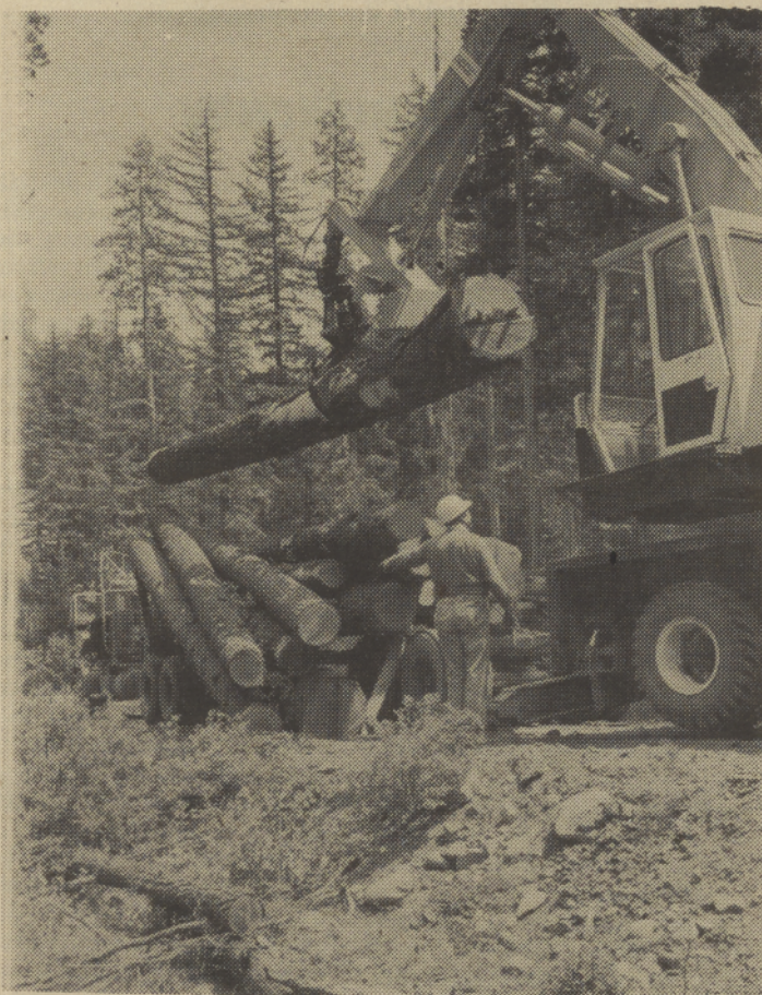
DRIVING A LOG TRUCK is a dangerous job and this is an example of what can happen. The stake broke on George Picard's truck as he rounded a bend, causing part of his load to come tumbling down. A very unhappy George is inspecting the damage, while the loader unloads the shifted logs.
