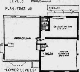
HOW A SPLIT-LEVEL puts basement space to work by raising part of it to grade level. This house has a built-in garage, a big recreation room with sliding glass doors to garden terrace, and an extra lavatory on the lower level. The house covers only 1,338 square feet. This is plan 7542AP by Herman H. York, architect, 90-04
