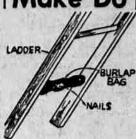
To Prevent slipping on the rungs of a ladder when work-ing in a muddy area, wrap a burlap bag around the bottom rung. This makes it easy to wipe your shoes on the bag and possibly avoid a serious accident. It's a tip from the American Builder's pool of
