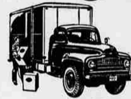
For bulky loads! The medium-duty L-160 series with van body means ease of handling and exceptional cab comfort. GVW's 14,000 to 16,000 lbs.
