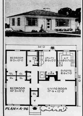
utility room replacing basement. Economical to build, this house calls for an insulated floor slab laid on gravel fill. This is Plan A-96 by the Small House Planning Bureau, St. Cloud, Minn. It covers 952 square feet and contains 10,472 cubic feet.
