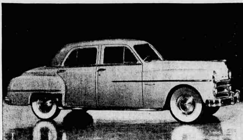
New Dodge Coronet Four-Door Sedan —New body lines, larger rear window and fresh front end styling identify the new Dodge Coronet four-door sedan. The new Dodge line consists of 10 body styles on two wheelbases. Coronet models, on a 123 1/2-inch wheelbase, are available with Gyro-Matic transmission, which frees the driver from shifting. Fluid drive is standard equipment on all Dodge cars. Stan Baker Motors are the Salem Dodge dealers.
