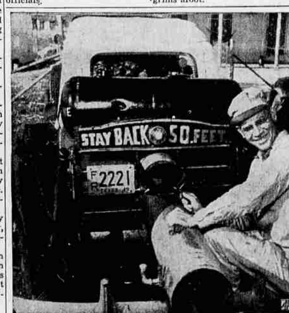
Jetmobile—Exhaust stacks are shown protruding from a jet turbine and a ram jet engine mounted in the rear of an old model car by John R. Mitchell (shown kneeling), a Chance-Vought aircraft employe at Dallas, Tex. Mitchell says his jetmobile costs only two-tenths of a cent per mile to operate, and is capable of generating 800 pounds of thrust, equal to about 200 miles an hour. But Mitchell explains it isn't practical for city driving, "it makes too dangd much noise." (AP Wirephoto)
