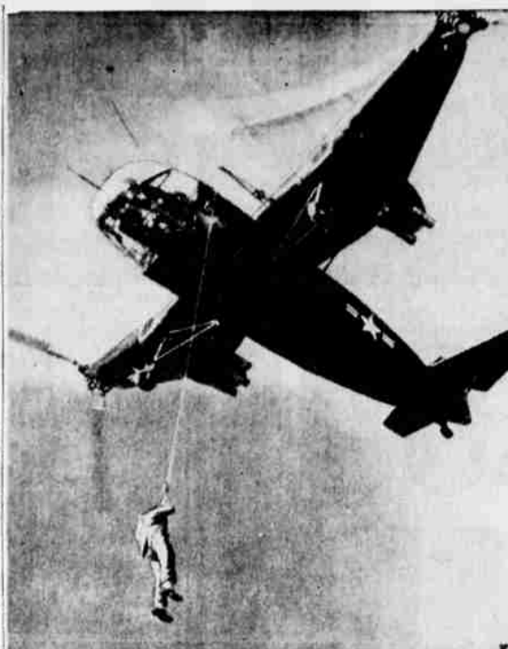
New Rescue Plane —Air rescue tests employing the McDonnell Aircraft Corp. XHJD-1 "Whirlaway," believed to be the first twin-engine, twin-rotor helicopter, have been successfully completed. The plane, a navy experimental helicopter, was tested for the purpose recently by air force representatives at Lambert-St. Louis field. In photo, Ralph Ballard, an experimental mechanic at the McDonnell plant has been lifted from ground and is about to be taken into plane. (AP Wirephoto)
