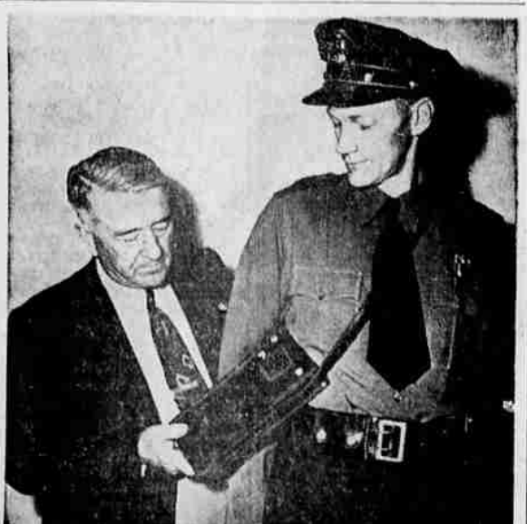
New Police Radio—Believed to be the first of its kind, this new radio receiver worn by Patrolman Floyd Lee is examined by Police Chief Charles Pray, of Portland, Ore. The radio, which may soon become regular equipment for Portland patrolmen, receives orders direct from police radio headquarters; calls are answered by telephone call box. (Acme Telephoto)
