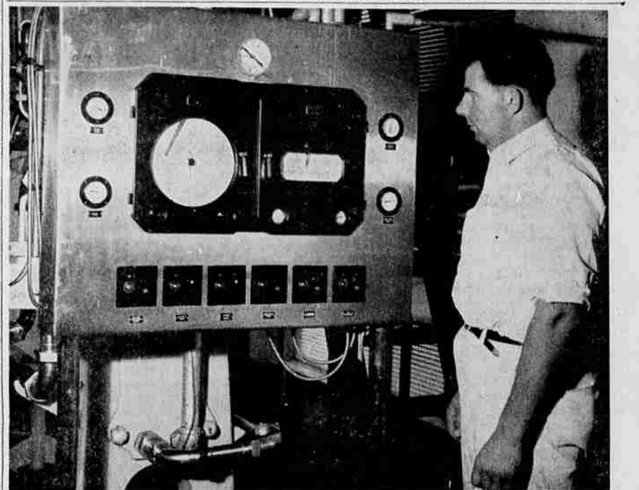
Smiling Loran Edlund the plant superintendent out at Curly's Dairy. The machine is the new pasteurizer that processes 4,000 quarts an hour. Edlund and his fellow workers at Curly's Dairy are now getting their Sundays off, just like ordinary people, all because of the cooperation of customers who are willing to accept a double order on Saturday and store the milk for one day in their own refrigerator. It's mighty nice to spend Sunday with our family and friends," says Loran.—(Adv.)
