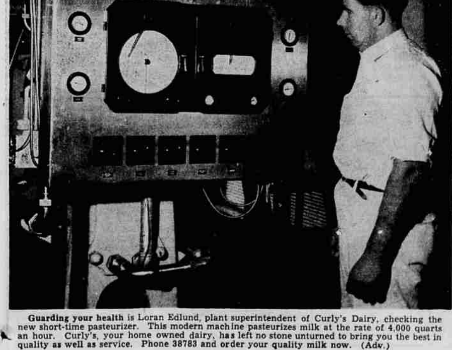
Guarding your health is Loran Edlund, plant superintendent of Curly's Dairy, checking the new short-time pasteurizer. This modern machine pasteurizes milk at the rate of 4,000 quarts an hour. Curly's, your home owned dairy, has left no stone unturned to bring you the best in quality as well as service. Phone 38783 and order your quality milk now. (Adv.)
