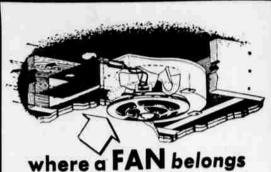
BLO-FAN electric ceiling ventilator builds in between the ceiling joists directly over the kitchen range -
