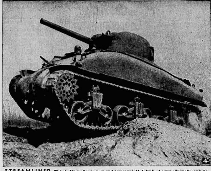
STREAMLINED—This is Uncle Sam's new and improved M-4 tank. Lower silhouette and abrupt angles make it a more difficult target. Turret holds a 75 mm. gun.
