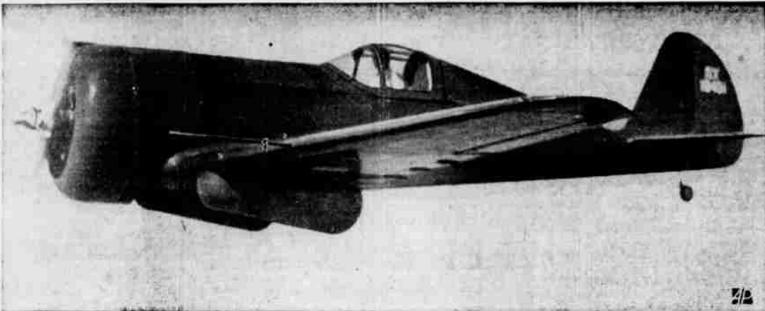
OUT OF SIGHT IN RECORD TIME, this new 4,000-lb. attack plane can reach 5,000 feet in 1.5 minutes, 20,000 feet in less than 6 minutes. Twin machine guns in the nose fire through propeller. Plane has duplex superchargers on 600-H.P. engine.
