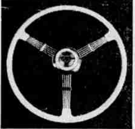
TENITE STEERING wheels of attractive spring steel spoke design are a style feature of the 1937 Buick cars. The Buick crest is carried in the center on the horn button.
