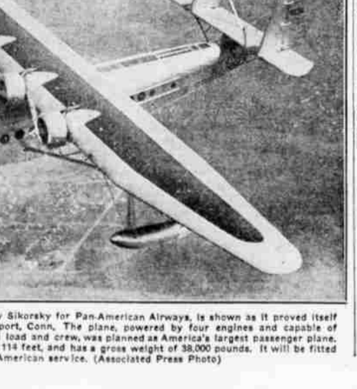
The plant flying boat B-42, built by Sikorsky for Pan-American Airways, is shown as it proved itself worthy on a test flight over Bridgeport, Conn. The plane, powered by four engines and capable of carrying 2,500 miles non-stop with a full load and crew, was planned as America's largest passenger plane.
