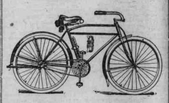
Note the "double construction" features throughout. Reinforced front forks, double bar frame, double spring
