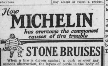
the tire are forced inward, subjecting them to a severe strain that tends to separate and break the cords.
