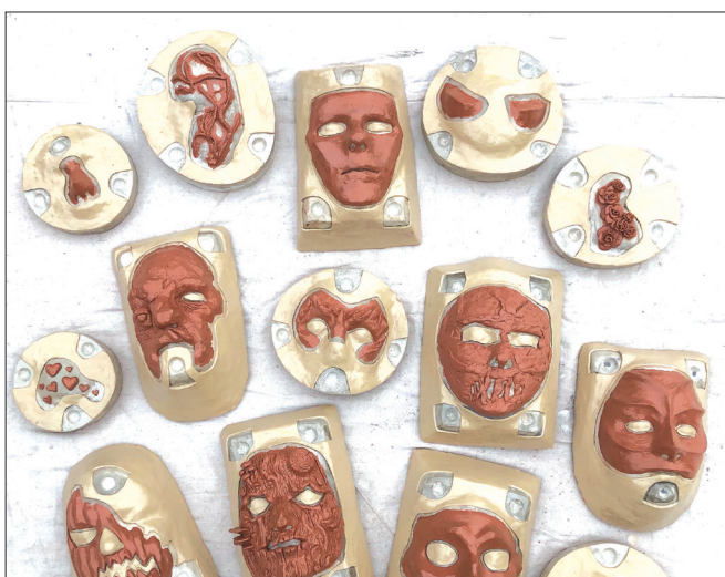
JR Rymut/Contributed Photo Clay character sculpt is affixed to plaster casts of the students' faces. When these are casted in another shell of plaster, the clay is scraped out and then silicone can be injected.
