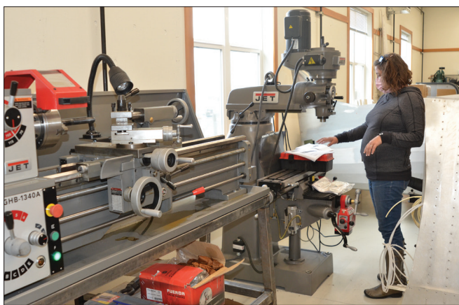
Bill Bradshaw/Wallowa County Chieftain A metal lathe, left, and a drill press are two of the machines aviation students learn to use in Lexi Rindfleisch's aviation classes at Joseph Charter School.
