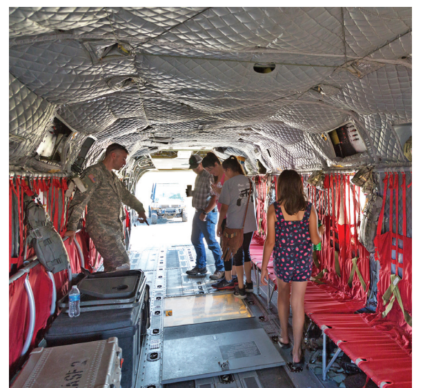
ABOVE Visitors peer down into the Chinook's viewport used to check the cargo that is being transported beneath the big chopper. The Chinook can transport up to 20,000 pounds of cargo, including Humvees that are slung underneath or stowed inside. The cheerful red upholstery accommodates 32 passengers.
