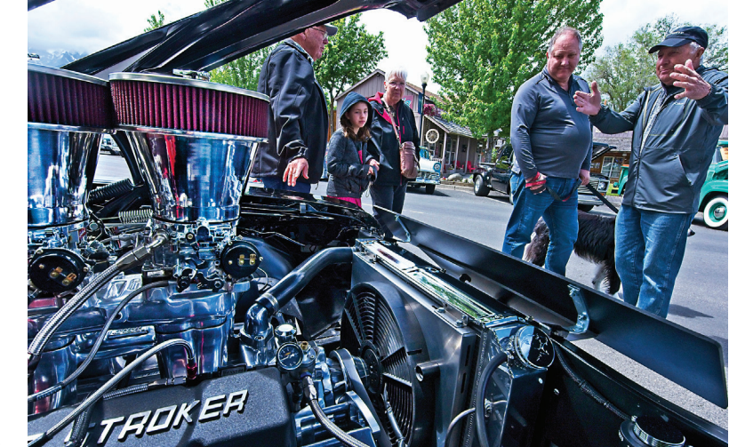
The 383 engine in Dominic Nation's 1972 Chevy Nova turns out 518 horsepower, and takes the vehicle from 0 to 122 mph in 11.8 seconds.
