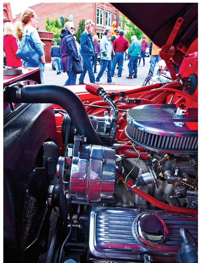
A 1949 Chevy 3100 pickup owned by Bret and Rhonda Paulson of Lewiston, Idaho, sports a 350 Crate engine with plenty of chrome. It also boasts rack and pinion steering from a 1989 T-bird, a 1991 Camaro rear end, and a DeSoto rear bumper.
