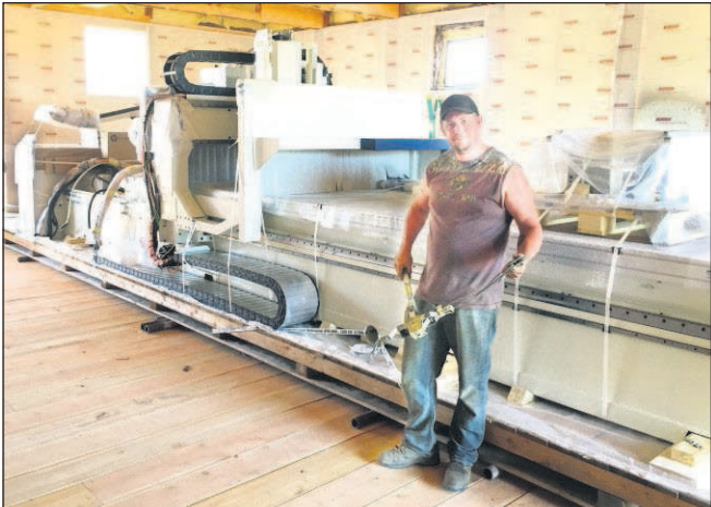
M. Crow & Co. employee Joey Haskins stands next to a new Computer Numerical Control machine, which is essentially a computer operated three dimensional router/carver. This machine, along with several other state-of-the-art woodworking machines, will soon employ up to seven people full-time making high-end walnut tables. Former Wallowa County resident Tyler Hays, a very successful artist/designer owns M.Crow & Co. and said he wants to provide Wallowa County residents with full-time jobs that pay real family wages.
